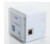
Ethernet socket (absent on WiFi device)
